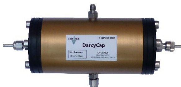
Fig. 3. Coreholder containing the 2 porous plates and the sample. The two outlet tubings are used to provide the electrical contacts.
