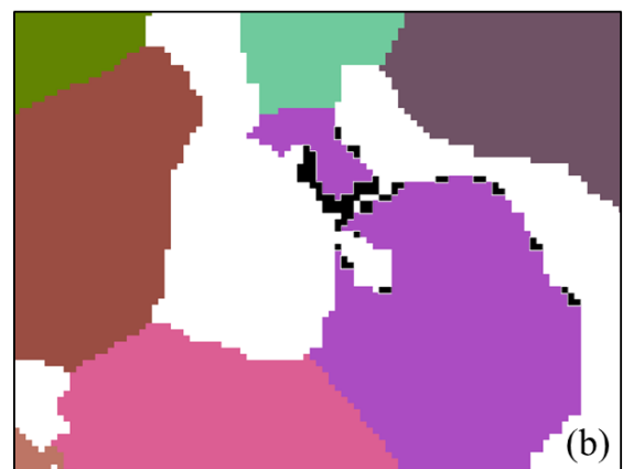
Fig. 8. Structural deformation for the sample of initial porosity = 23.82%: (a) pore shrinking and (b) throat necking. Black region indicates porosity change after applying stress.
