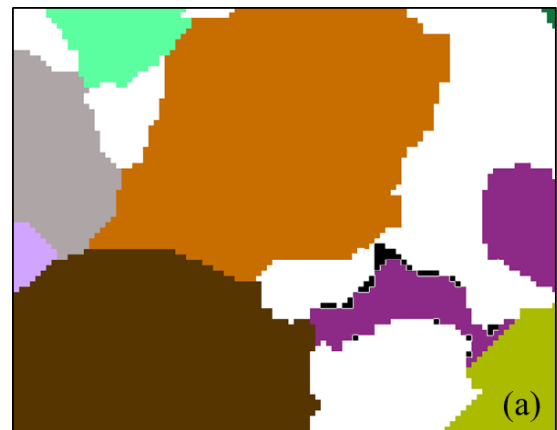
Fig. 7. Body deformation for the sample of initial porosity = 23.82%. Black region indicates porosity change after applying stress.
