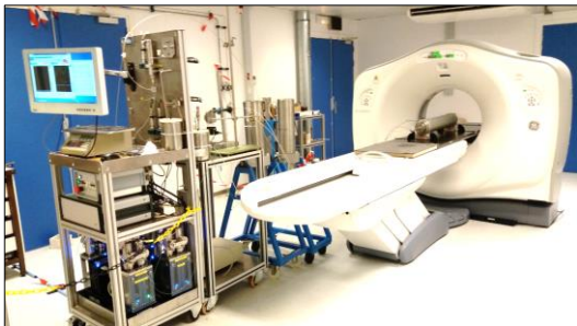
Fig. 1. Overview of the IFPEN medical CT Scan GEHC Discovery 750HD and the experimental setup
