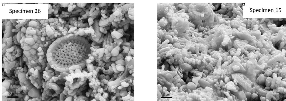
**Figure 4:** FEG-SEM micrographs of plug #26 (untreated) and plug #15 (treated with 5% Acidgen™ FG) showing a considerably larger number of grains in the fraction  $<1\ \mu\text{m}$  in the treated specimen.
