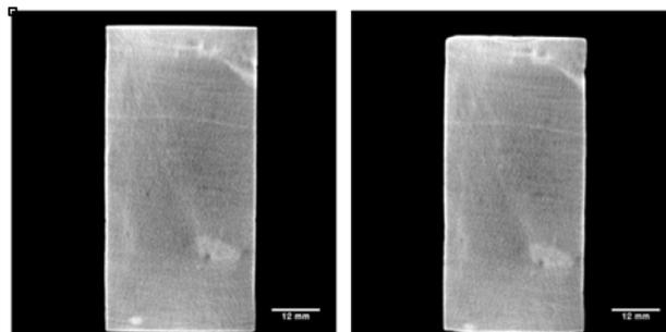
**Figure 5:** CT-images of plug specimen #57. A) Before treatment with 2% acetic acid. B) After 6 treatments with 2% acetic acid. Note that the specimen has become considerably smaller due to the treatment.
