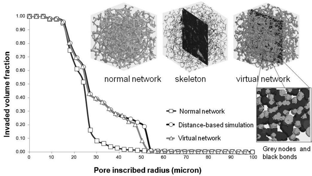
Figure 7. Filling curves for drainage into the mixed porous system shown in Figure 6, from network flow simulation on “normal” and “virtual” networks, as well as from a distance-based simulation.
