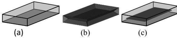
Figure 1. Using normal grassfire transformation, a 3D object (a) can be shrunk to a medial surface (b) in comparison with our targeting fracture surface (in black, (c)).
