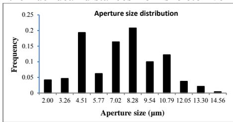
Figure 3. The aperture distribution of the fracture shown in Figure 2(a).
