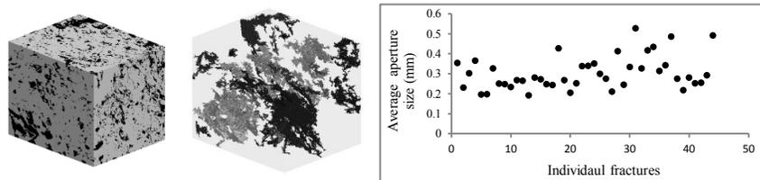
Figure 4. (a) A  $\mu$ -CT tomograph of a carbonate at resolution of 48  $\mu$ m and (b) the medial surfaces of 46 fractures in different grey levels, (c) a scatter plot of average apertures for the fractures.
