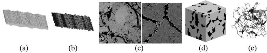
Figure 2. An artificial fracture (a) and its medial surface (b), carbonate rocks with fractures (c), sandstone image (d) and its skeleton (e). The different grey levels in (b) and (e) to represent the distribution of the Euclidean distances from skeleton voxels to their closest solid voxels.
