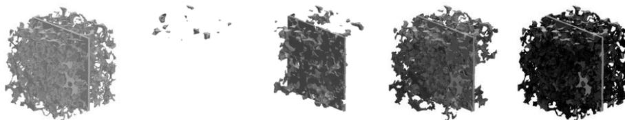
Figure 6. A mixed porous system embedded with an artificial fracture. And visualisation of distance-based simulation of drainage (downwards), showing the non-wetting phase varying from large pores (light grey) to small pores (dark grey).
