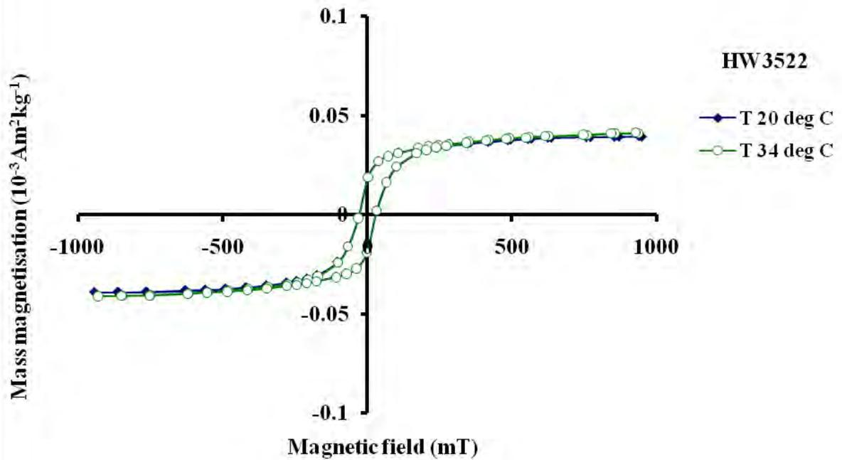
Figure 3. The extracted ferrimagnetic hysteresis curves at various temperatures for sample HW3522.
