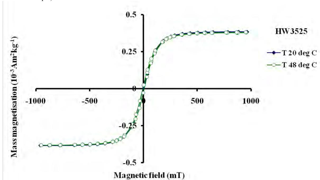
**Figure 5.** The extracted ferrimagnetic hysteresis curves at various temperatures for sample HW3525.
