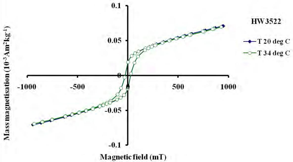
Figure 2. Magnetic hysteresis curves at two different temperatures for sample HW3522 (a sediment).
