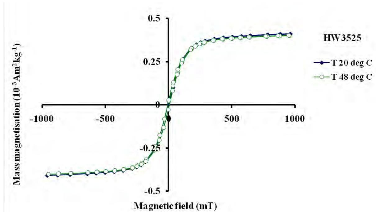
**Figure 4.** Magnetic hysteresis curves at two different temperatures for sample HW3525 (a crystalline basement sample).
