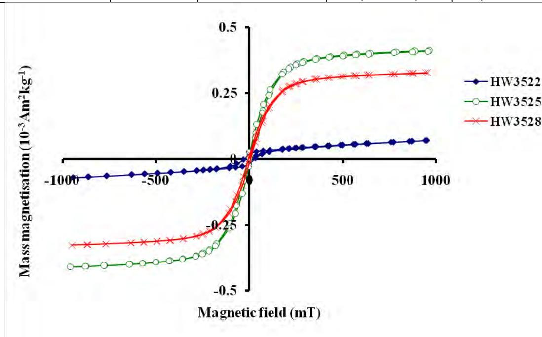
**Figure 1.** Ambient (room temperature) magnetic hysteresis curves for three powdered rock samples from the Hunt Well in northern Alberta.
