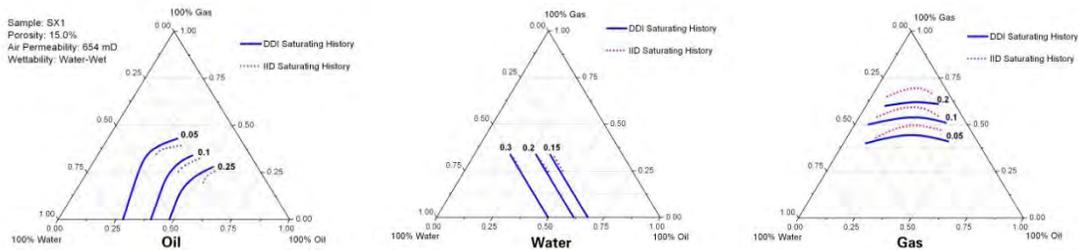
**Figure 2. Isoperms of Water, Oil and Gas for Water-Wet Core SX1**
