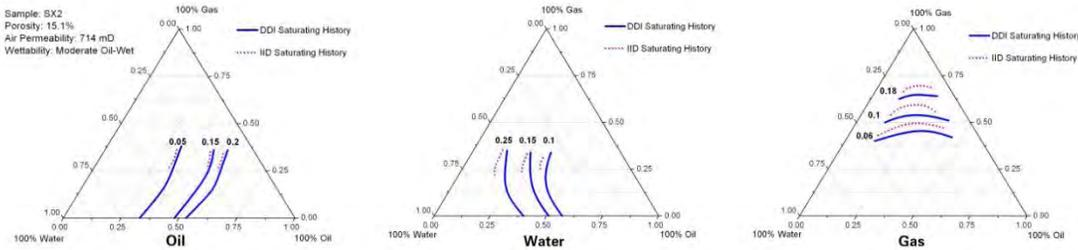
**Figure 3. Isoperms of Water, Oil and Gas for Oil-Wet Core SX2**
