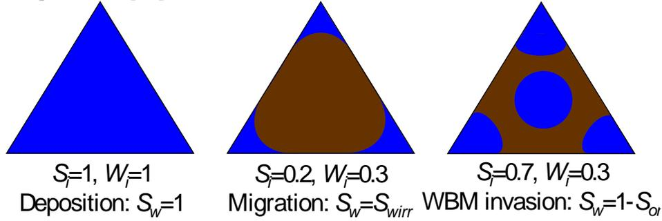
Figure 3: Schematic representation of the different states of a triangular pore after deposition (left), oil migration (middle), and flushing caused either by WBM (Water Based Mud) filtrate invasion or water injection (right).  $S_i$  is defined as the volume fraction of water in that  $i^{\text{th}}$  pore (bound by  $0 \leq S_i \leq 1$ ), while  $W_i$  is the surface fraction of the pore wall that is wetted by water (bound by  $0 \leq W_i \leq 1$ ).
