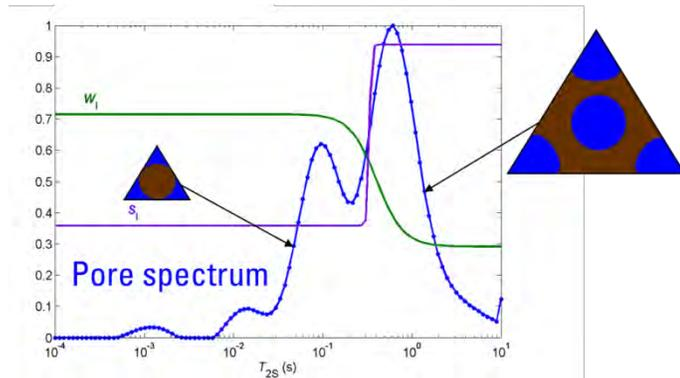
Figure 4: A representative example of the forward model and inversion output.  $S_i$  (purple line) and wettability  $W_i$  (green line) across the pore spectrum data (blue dots). The pore cartoons illustrate how the big pores (right) would look according to  $S_i$  and  $W_i$ , and similarly for the small pores (left). Note that the pore cartoons are meant as an illustration and do not correspond to the precise values of  $S_i$ ,  $W_i$ , and pore size.
