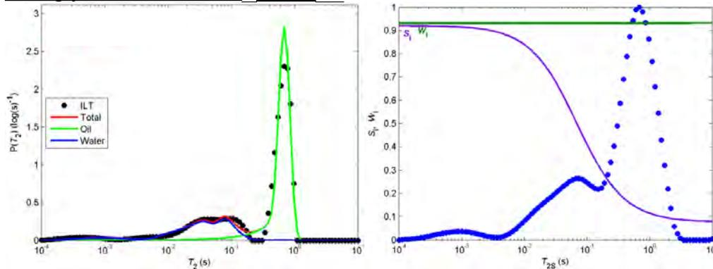
Figure 6: Same as Figure 5 but for a water wet plug at  $S_{wirr}$ . The saturation steps at which the plug has been submitted are  $S_W=1 \rightarrow S_{wirr}$ . The overall water saturation is  $S_{NMR} = 0.29$  and the wettability index is  $I_{NMR} = +0.86$ .
