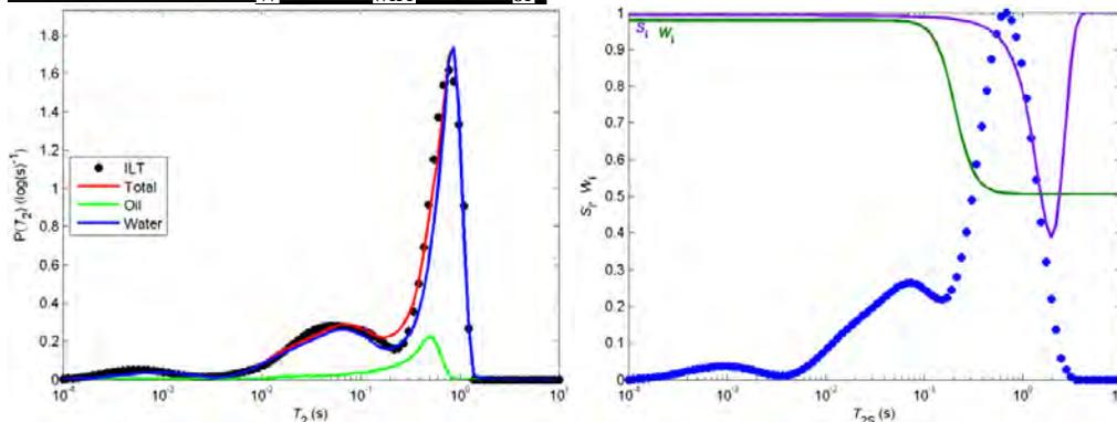
Figure 7: As Figure 5 but for a water wet plug at  $S_{or}$ . The saturation steps at which the plug has been submitted are  $S_W=1 \rightarrow S_{wirr} \rightarrow (1-S_{or})$ . For this solution the overall water saturation is  $S_{NMR} = 0.89$  and the wettability index from  $I_{NMR} = +0.32$ .
