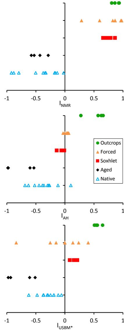
Figure 8: Different wettability indices (x axis) as a function of the sample preparation (y axis): native state (empty blue triangles), aged cores (black diamonds), soxhlet cleaned (red squares), forced cleaned (full orange triangles) and outcrops (full green circles). Wettability index from (top) NMR, (middle) Amott-Harvey, and (bottom) USBM\* are shown.
