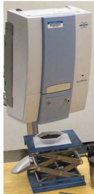
Figure 2. Mounted spectrometer setup for ease of collecting measurements.
