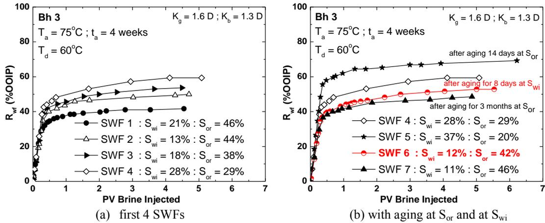
**Figure 3.** Oil recovery by SWF for Core Bh 3 (a) for the first 4 SWFs and (b) SWFs 4-7 for aging periods of 14 days at  $S_{or}$  at the end of SWF 4, 8 days at  $S_{wi}$  for SWF 6, and 3 months at  $S_{or}$  after SWF 6.
