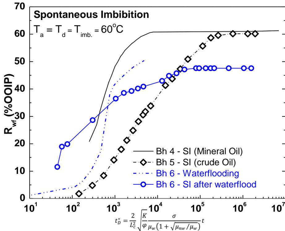
**Figure 9:** Recovery of WP crude oil by spontaneous imbibition for a core which had not been previously waterflooded (Bh 5) and a core which had been previously waterflooded once (Bh 6) including comparison with time for waterflooding for Bh 6.
