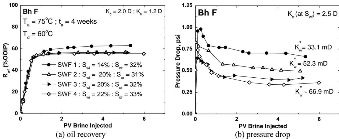
**Figure 5.** Recovery of WP crude oil and pressure drop vs. PV of seawater injected for 4 SWFs for fired and acidized Bentheim sandstone.
