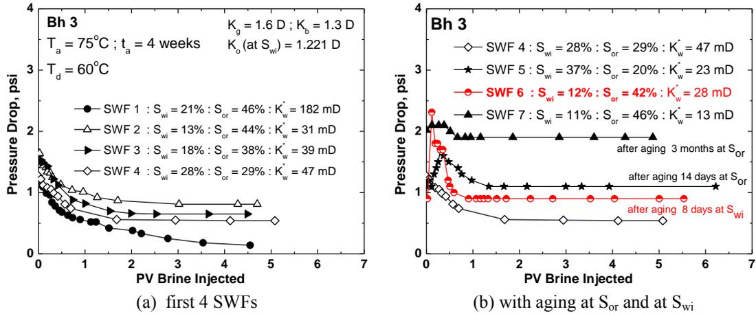
**Figure 4.** Pressure drop vs. PV injected for 7 SWFs.
