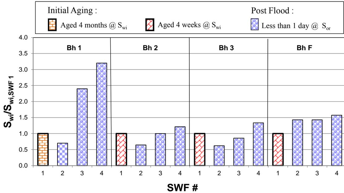
**Figure 6.** Summary of relative change in initial water saturation for the first four SWFs on each Bentheim core with  $S_{wi}$  normalized with respect  $S_{wi}$  for SWF 1.
