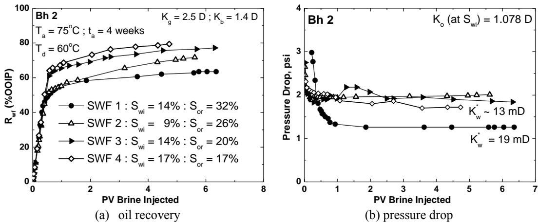
**Figure 2.** Oil recovery and pressure drop vs. PV injected for Core Bh 2 for four SWFs.
