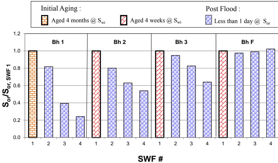
**Figure 7.** Summary of relative change in residual oil saturation for the first four SWFs on each Bentheim core with  $S_{or}$  normalized with respect  $S_{or}$  for SWF 1.
