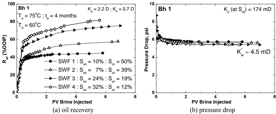
**Figure 1.** Oil recovery and pressure drop vs. PV of seawater injected for Core Bh 1 for four SWFs. ( $t_a$  is the aging time and  $T_a$  the temperature;  $T_d$  is the displacement temperature)
