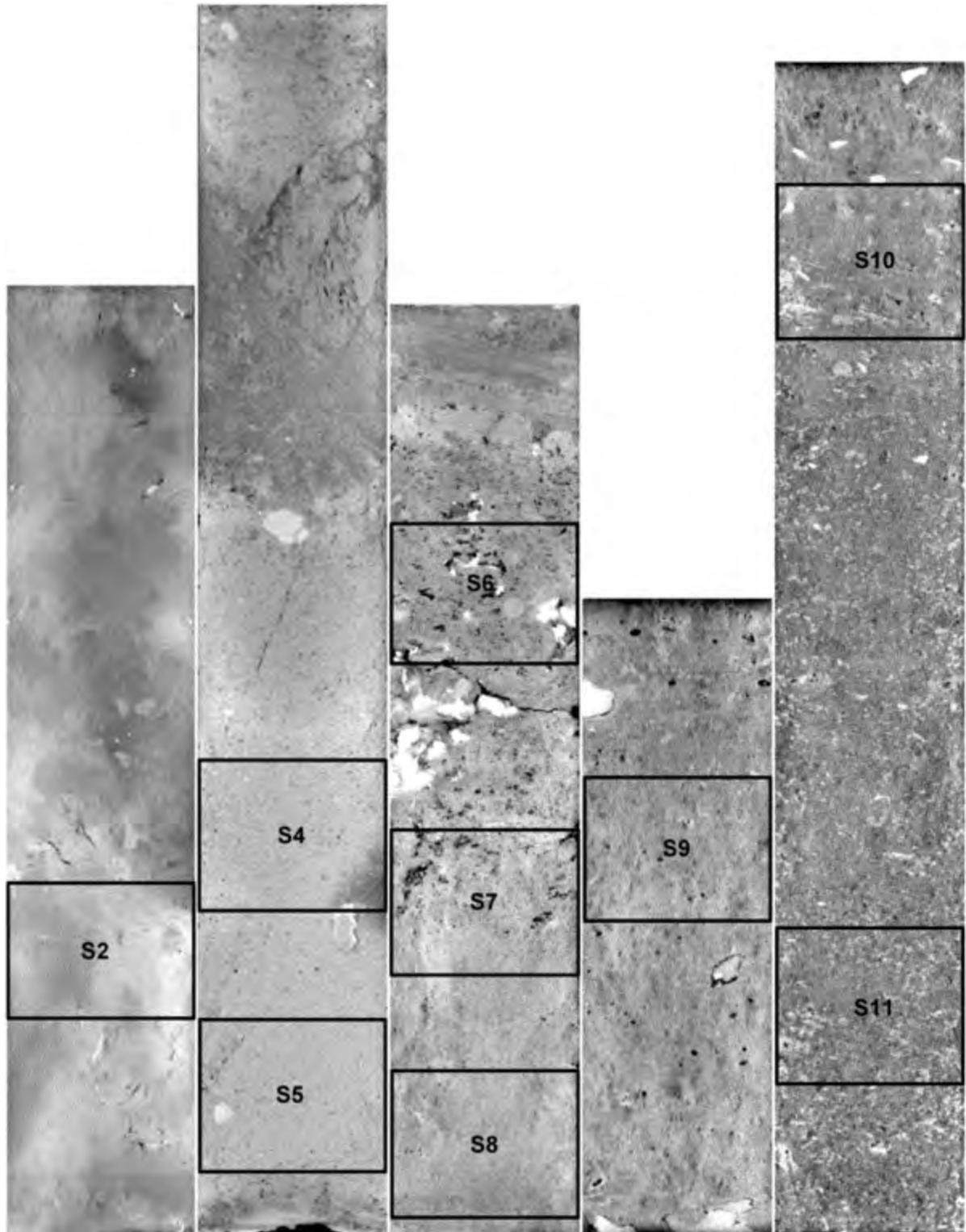
*Figure 2. Virtual slab surface extracted from the whole core tomograms, showing the different rock textures and the location of the FD core samples.*
