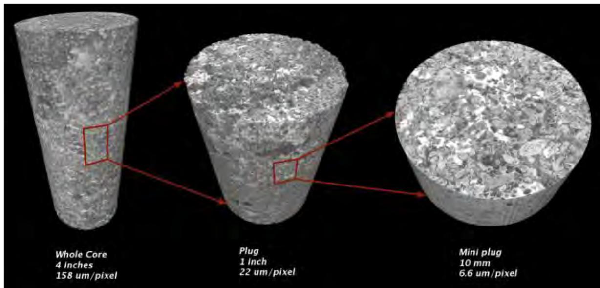
*Figure 1. 3D rendering of the tomogram for core plug S11C (middle), the corresponding whole core section tomogram (left), and an internal region tomogram (right), showing the rock texture heterogeneity at three scales.*
