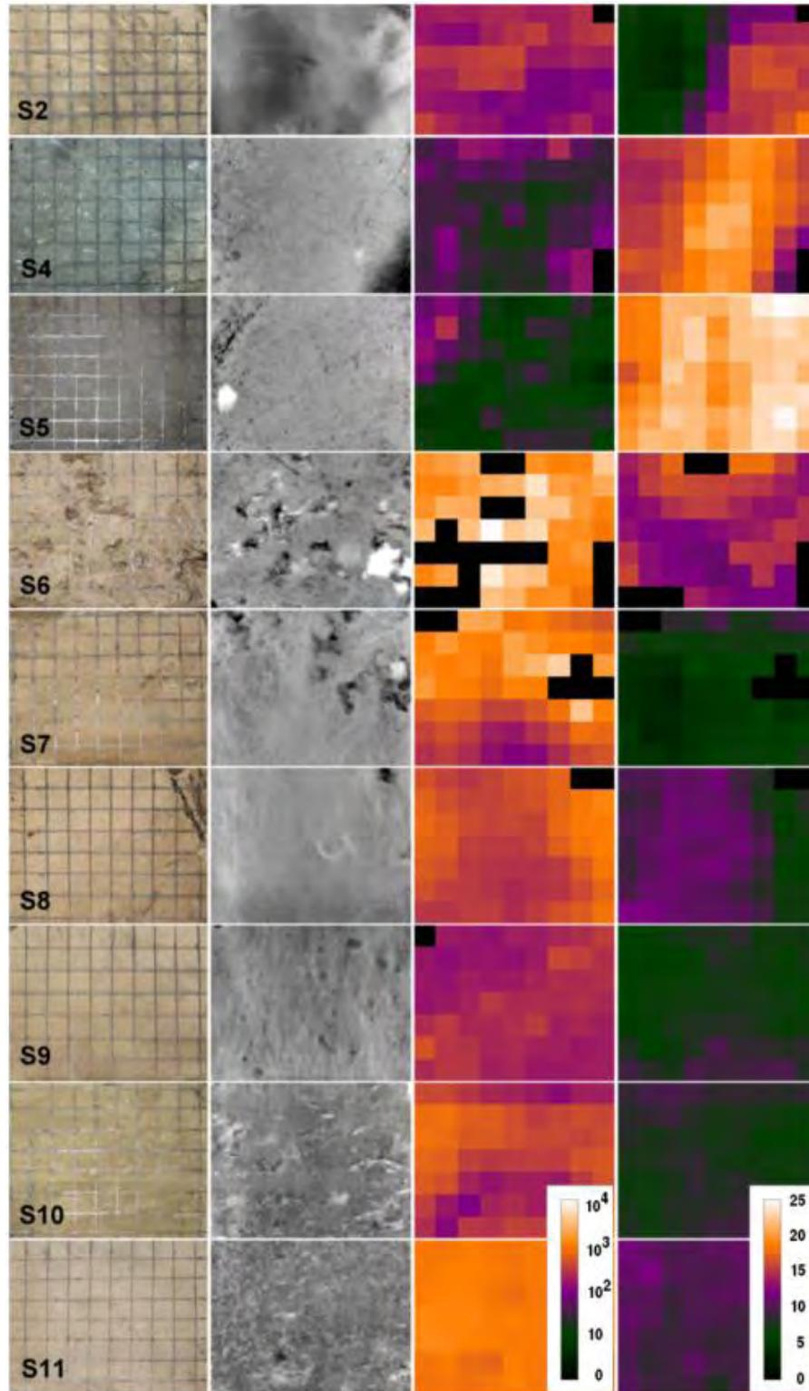
**Figure 3.** Slab surface of each FD cores (top to bottom) shown as (from left to right): picture, CT image averaged on 1cm thick, mini-permeability (mD), and resistivity (ohm-m), both measured in a grid of 1cm spacing, and scaled to a color map in log scale as shown.
