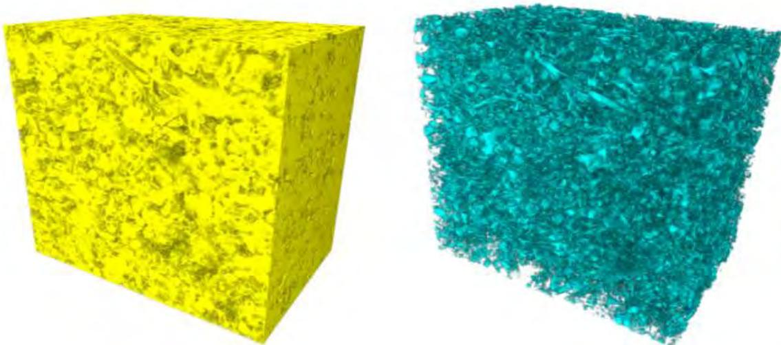
**Figure 8.** Rendering of the volume (about 0.5cm<sup>3</sup>) used on the simulation. The segmented solid phase (left) and pore phase (right) are shown. Porosity segmented at this resolution is about 17%, while the total porosity measured in the plug is 32%. The unaccounted porosity is below the image resolution and is assumed impermeable.
