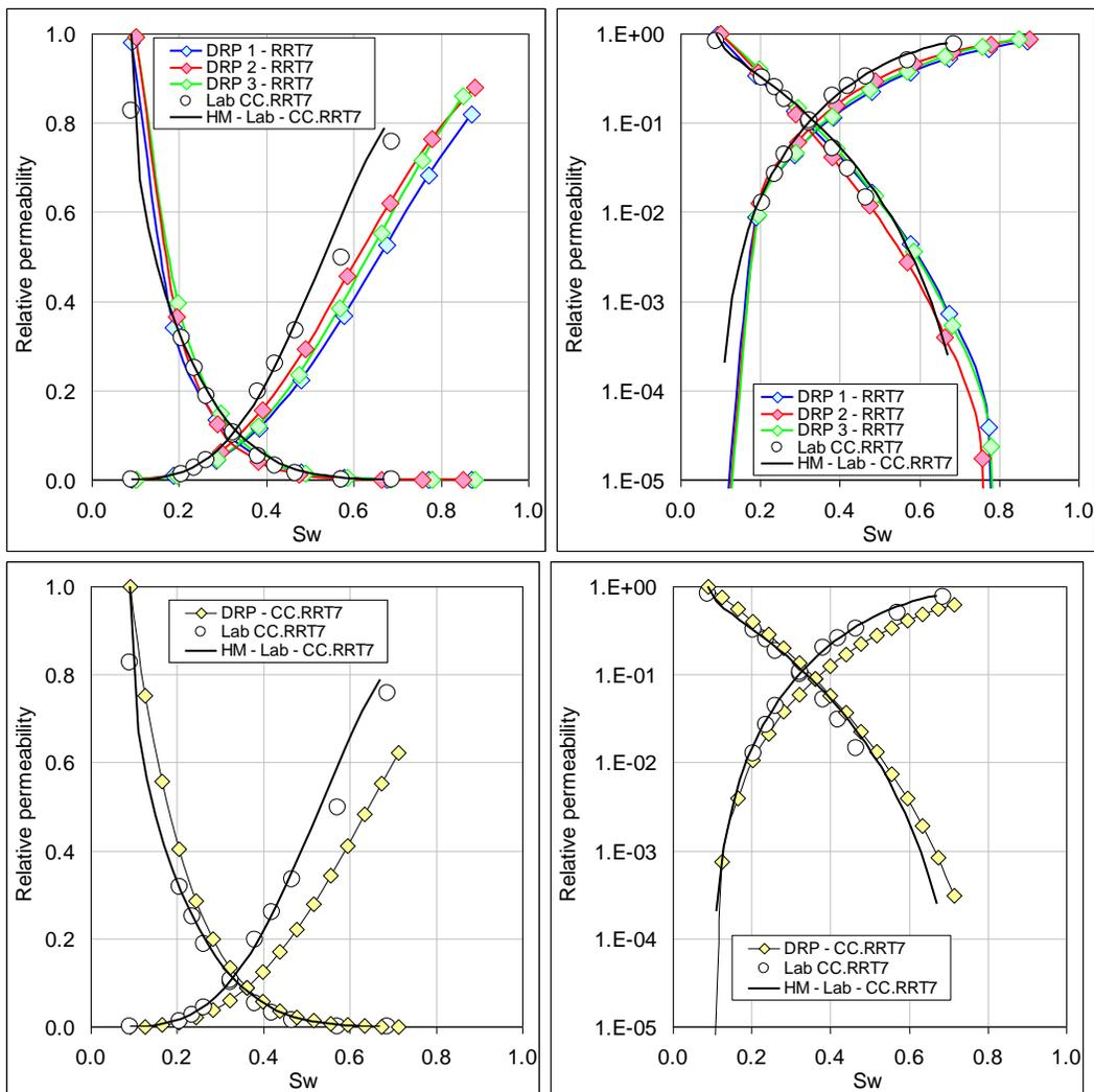
Figure 2: DRP and steady state test Relative permeability for RRT 7
