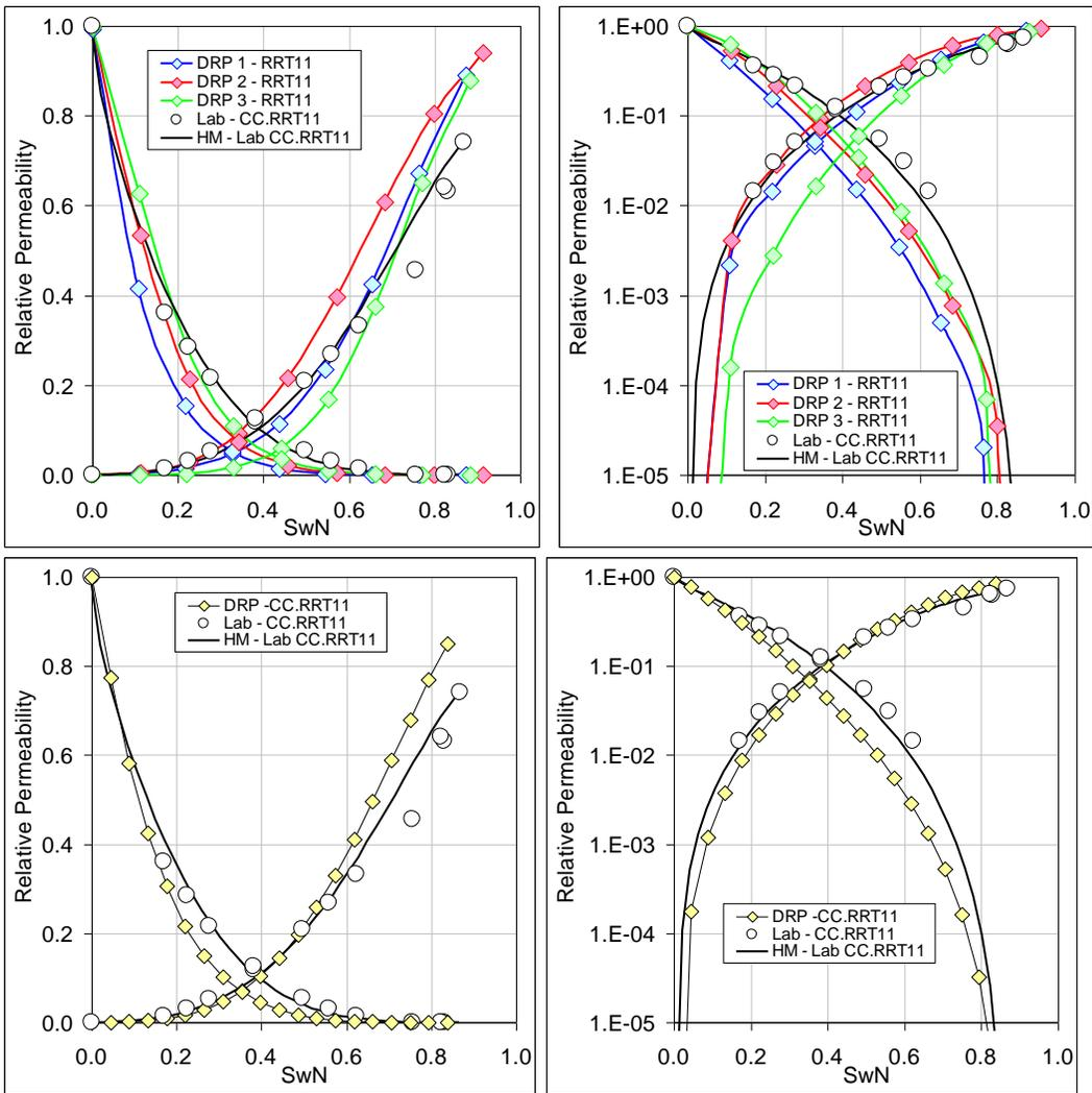
Figure 5: DRP and steady state test Relative permeability for RRT 11
