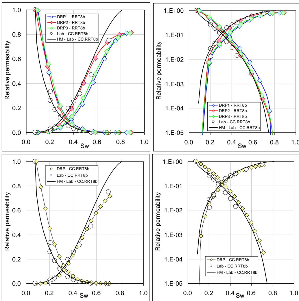
Figure 4: DRP and steady state test Relative permeability for RRT 8b
