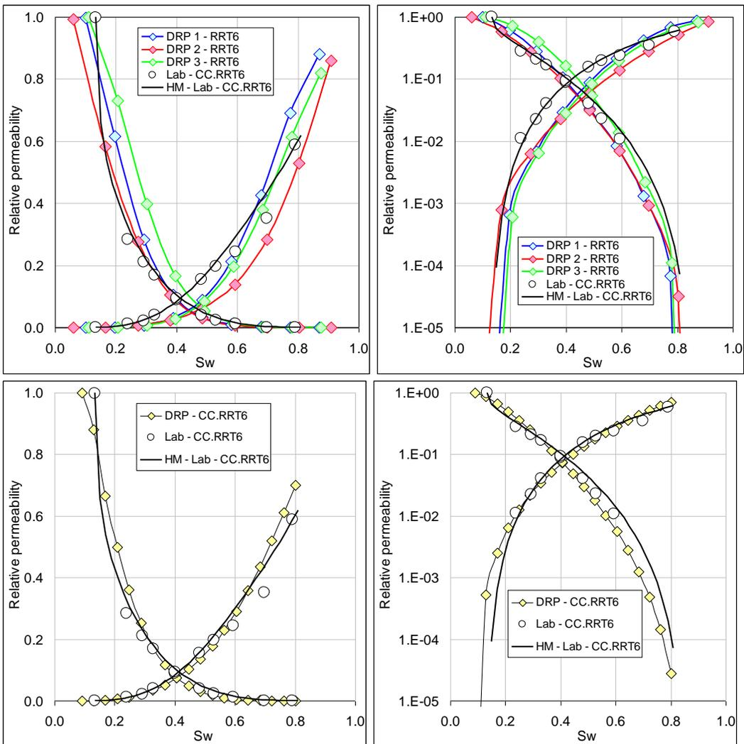
Figure 1: DRP and steady state test Relative permeability for RRT 6
