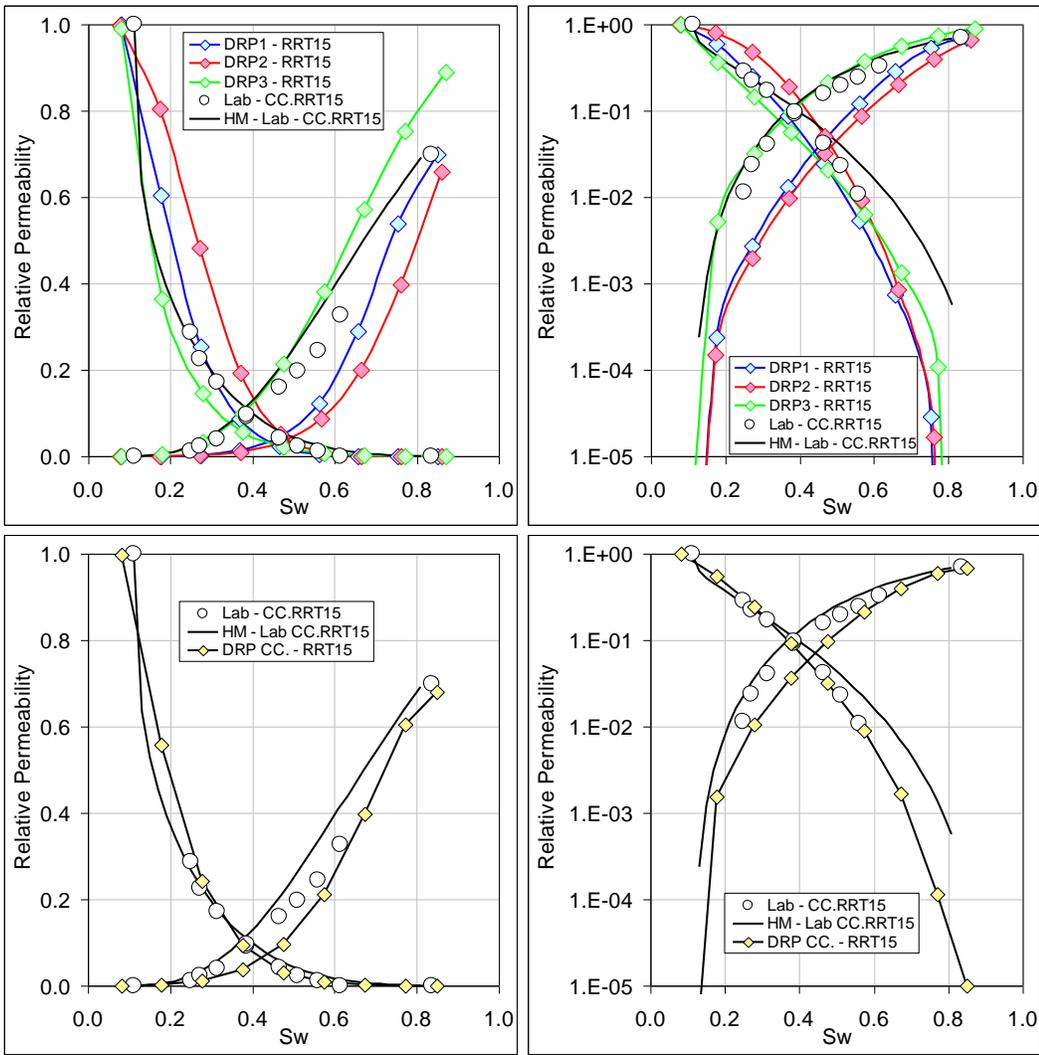
Figure 6: DRP and steady state test Relative permeability for RRT 15
