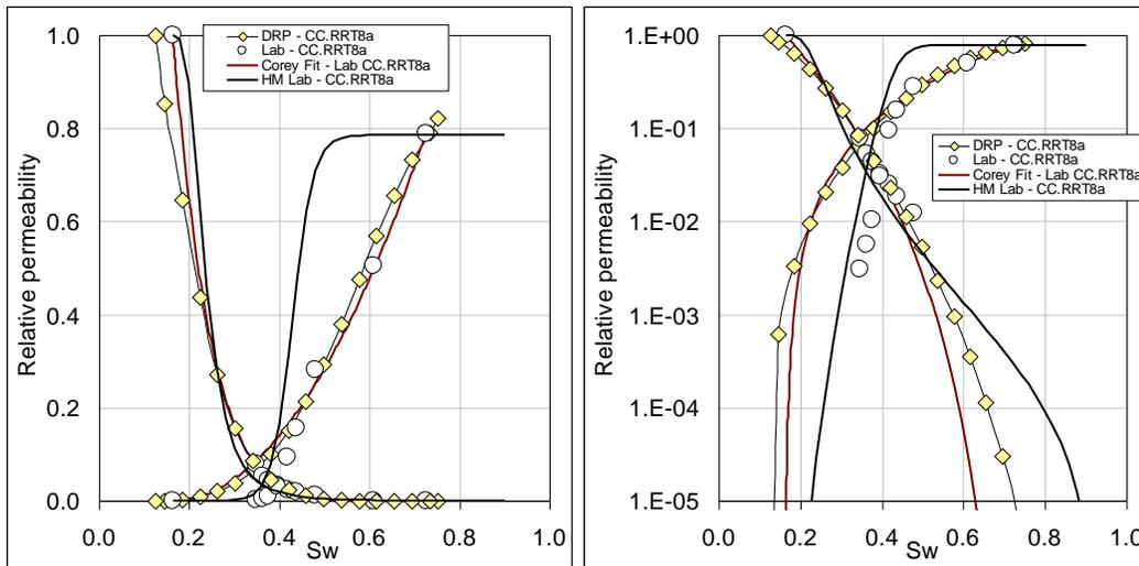
Figure 3: DRP and steady state test Relative permeability for RRT 8a
