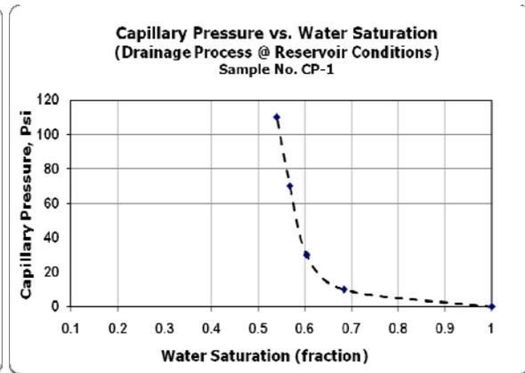
Figure 3) measured drainage capillary pressure vs. water saturation of sample CP-1 at reservoir conditions.
