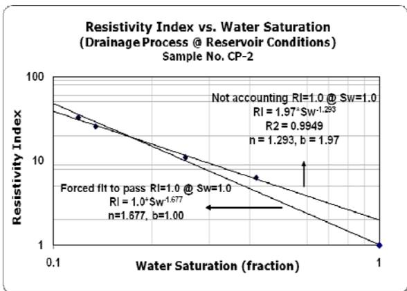
Figure 4) measured resistivity index values vs. water saturation of sample CP-2 from drainage process and two fitted regression curves.
