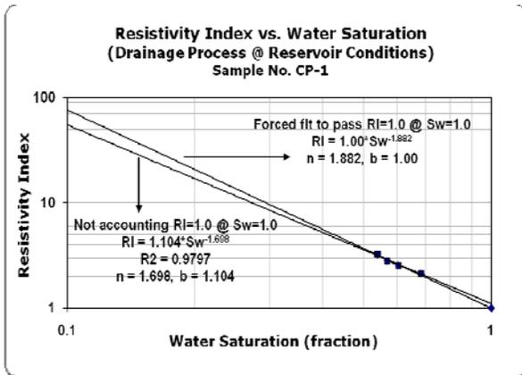
Figure 2) measured resistivity index values vs. water saturation of sample CP-1 from drainage process and two fitted regression curves.
