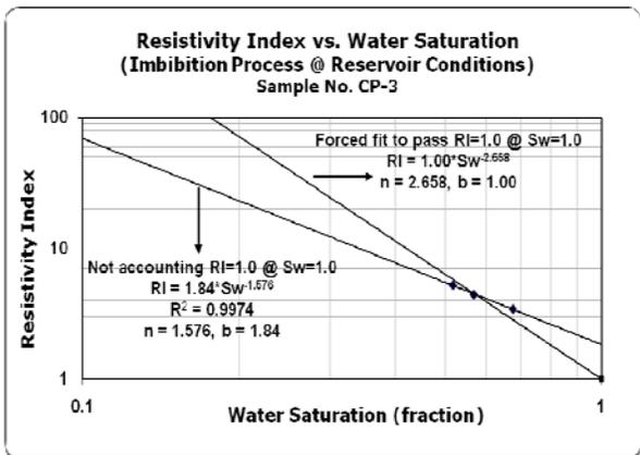
Figure 6) measured resistivity index values vs. water saturation of sample CP-3 from imbibition process and two fitted regression curves.
