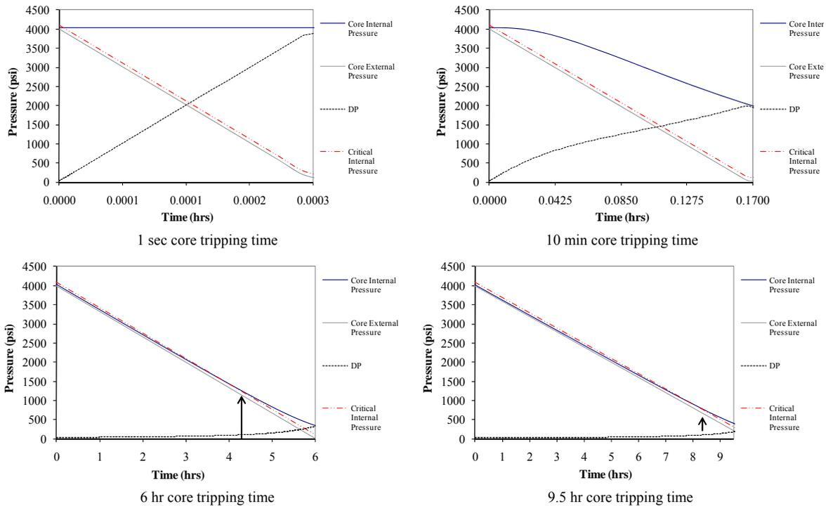
Figure 4. Internal-external pressures and DP versus time for a core of 0.001 mD
