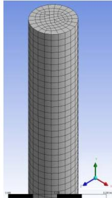
Figure 1 Representation of a fluid region of porous media flow discretized into a finite set of control volumes (mesh)
