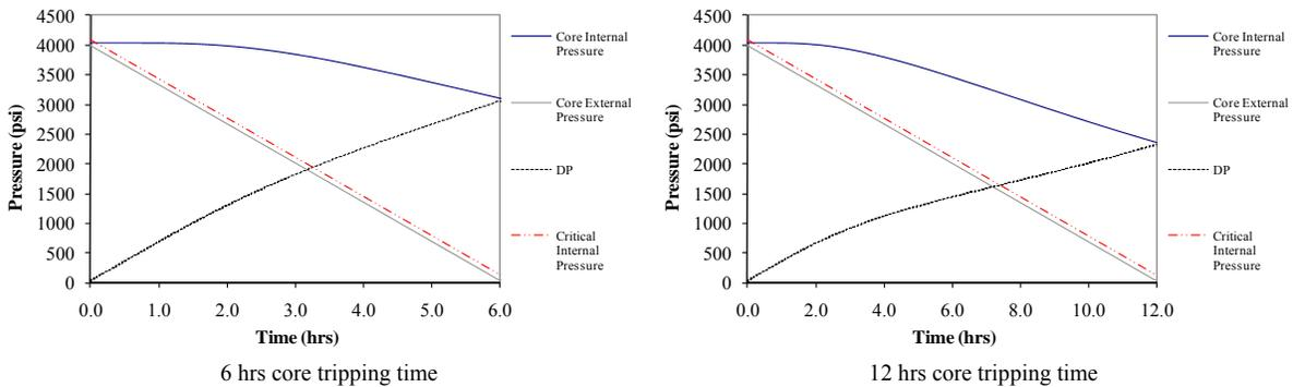
Figure 5. Internal-external pressures and DP versus time for a core of 0.00001 mD
