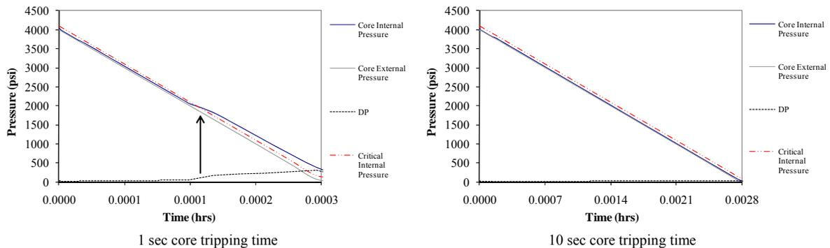
Figure 3: Internal-external pressures and DP versus time for a core of 300 mD
