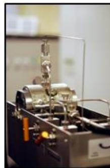
Figure 3: Photograph showing purge lines and injection ports connected to chamber
