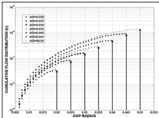
**Figure 5:** Example of cumulative flow distribution in the gaps region. The arrows indicate the value of  $I(r)$  for different values of radius of strained particles ( $r_s$ ).
