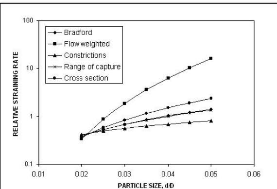
**Figure 6:** Correlation between straining constant and particle size calculated with five different methods. The flow-weighted method gives the largest deviation with respect to the other methods.
