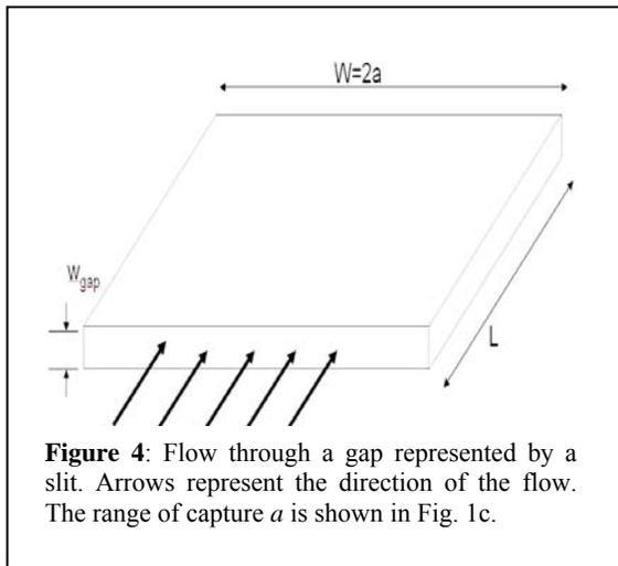
**Figure 4:** Flow through a gap represented by a slit. Arrows represent the direction of the flow. The range of capture  $a$  is shown in Fig. 1c.
