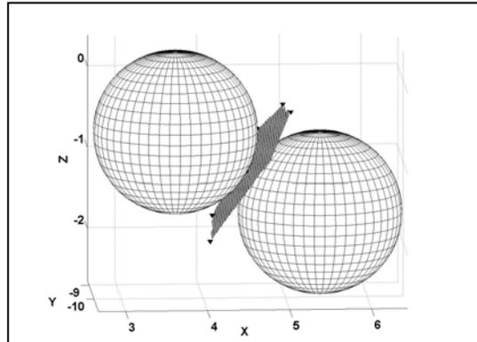
**Figure 3:** Spatial view of two spheres in Finney packing. The centers of the Delaunay cells ( $\blacktriangle$ ) in which the spheres are contained and the center of the gap between the two spheres lie in the same plane.
