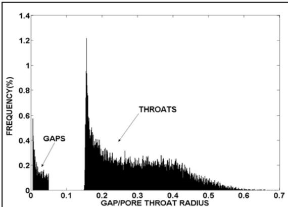
**Figure 2:** Frequency distribution of gaps in the size range of interest for anomalous straining and pore throats in Finney packing. Gap radius equals half gap width.
