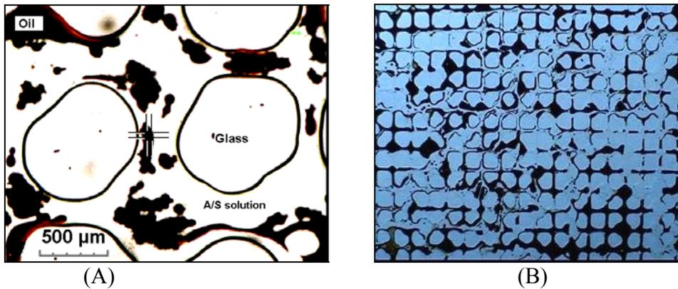
Figure 4. Emulsification and entrainment of heavy oil in water phase in micromodel test. A) pore-level image, B) image of micromodel during oil displacement.
