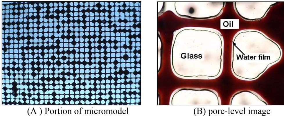
Figure 1. Micromodel with heavy oil and irreducible water saturation.
