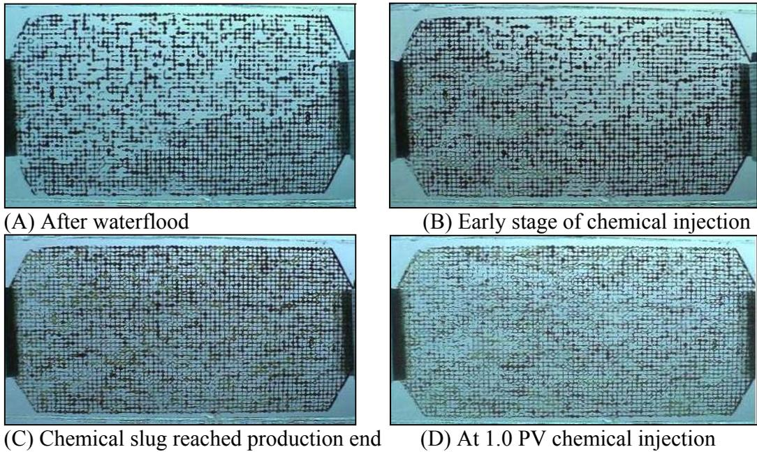
Figure 5. Pictures of micromodel test with alkaline injection.
