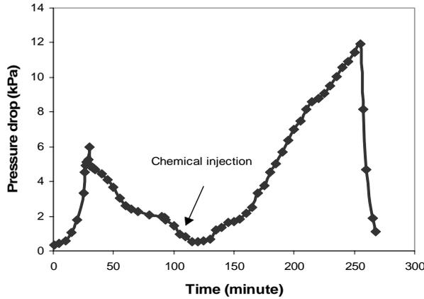
Figure 3. Pressure drop in water and alkaline flooding in a micromodel test.
