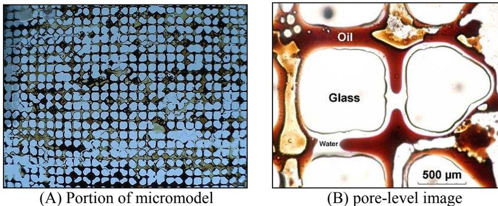
Figure 2. Formation of W/O emulsion in alkaline injection.
