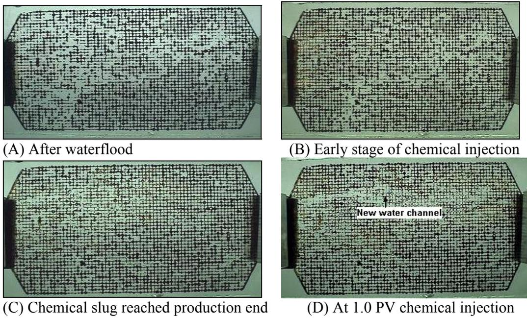
Figure 6. Photos of micromodel test with alkaline/surfactant injection.
