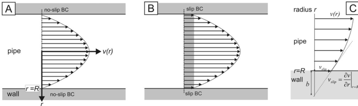
**Fig. 2:** Pipe flow with no-slip (A) and slip (B) boundary conditions. For slip the tangential velocity of the fluid at the wall is  $v_{slip} > 0$ . The slip velocity right at the wall  $v_{slip}$  can be derived from the slip length  $b$  which is defined via extrapolation of the velocity gradient into the wall (C).
