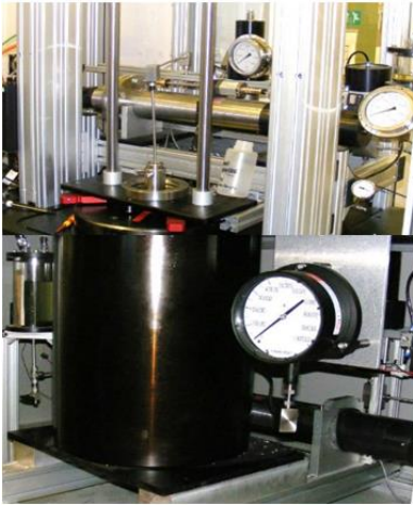
Figure 1. Picture and schematic diagram of the new porosimeter under confining stress.
