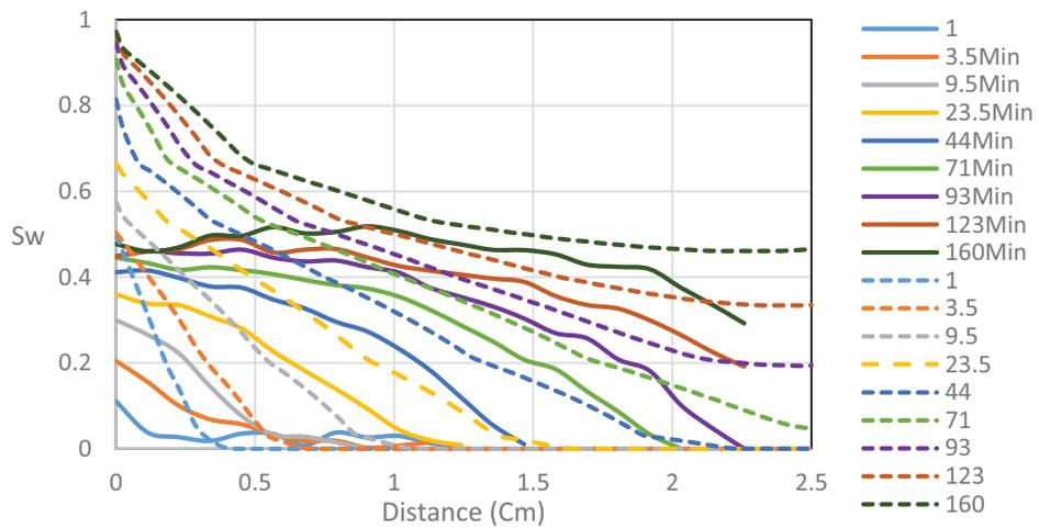
Figure 6: Comparison of the simulated (dash lines) and experimental (solid lines) saturation profiles for co-current spontaneous imbibition test
