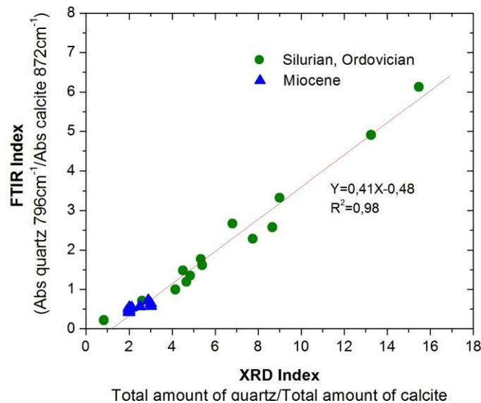
**Figure.2.** Correlation of FTIR and XRD results on the basis of quartz to calcite content ratio for mineralogical representativeness control of cuttings used for Vp/Vs tests.
