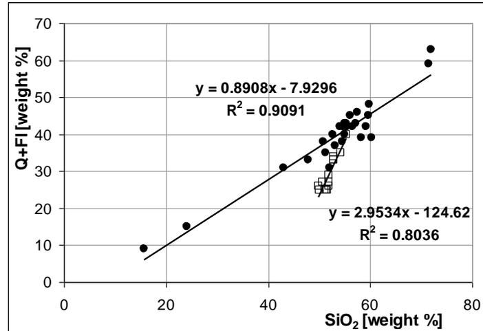
**Figure.1.** Correlation between the mineralogical and chemical indexes defined respectively as the sum of quartz and feldspars content and SiO<sub>2</sub> content. Blue diamonds – the Silurian – Ordovician set of data, pink squares - the Miocene set of data.
