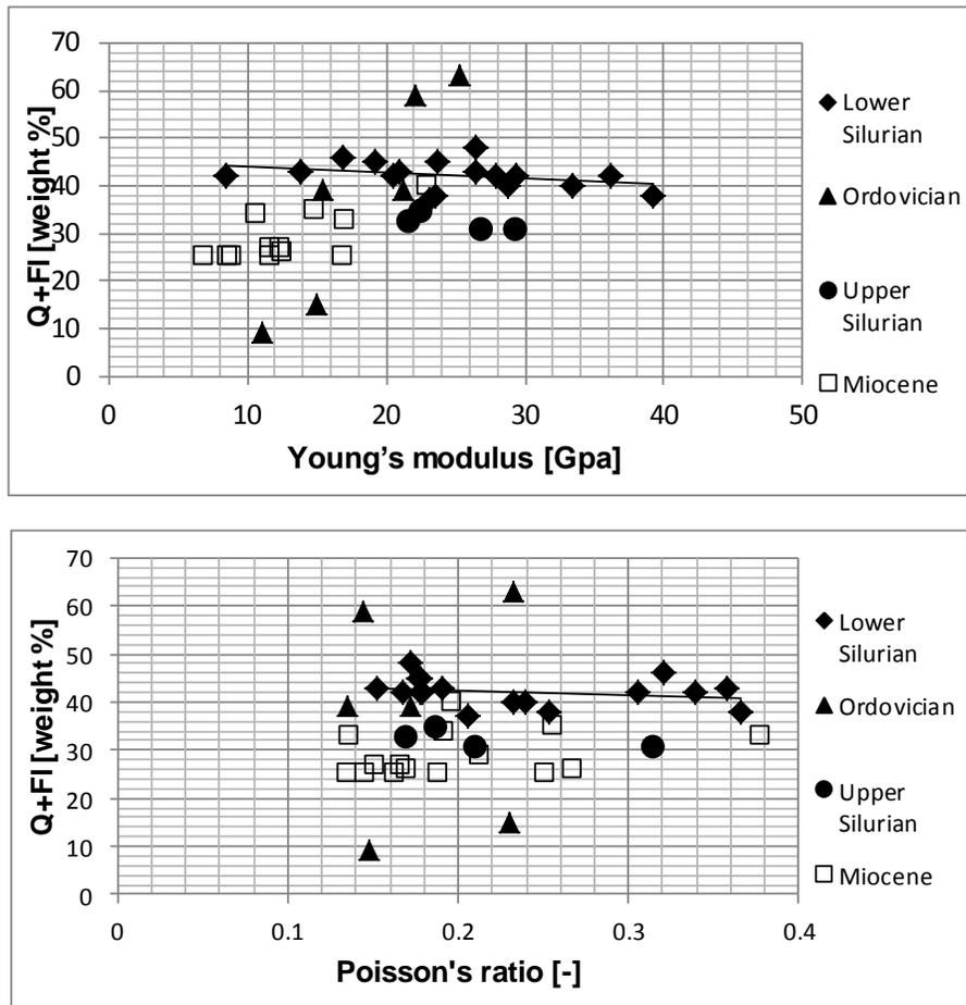
**Figure.4.** Relation between the mineralogical parameter of rock brittleness and the acoustic moduli: a) Young's modulus, b) Poisson's ratio.
